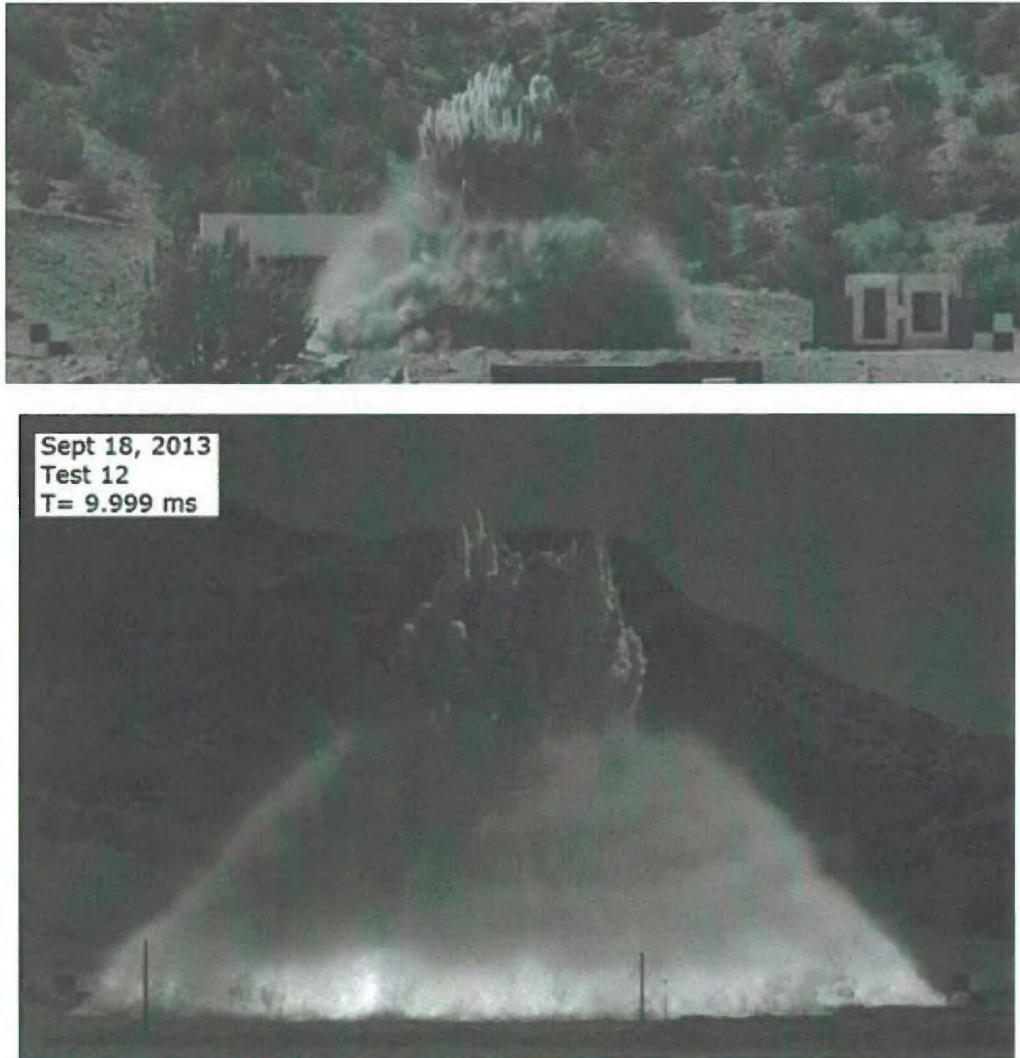
Figure 58: High speed video comparison at t = 10 ms post detonation for (top) 24/76 ANIP/AS and (bottom) 64.76/35.24 ANIP/dolomite mixtures respectively.
