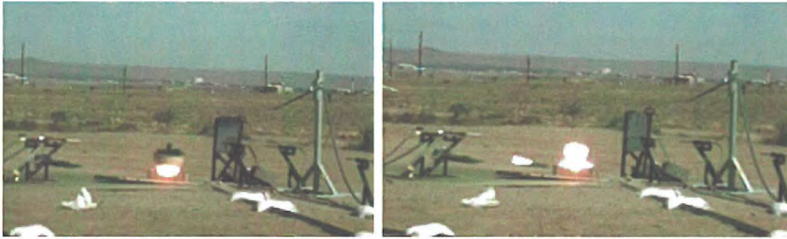
Figure 18: 0.8 lb of ██████/LH (left) and FGAN/LH (right) respectively at approximately t=156 μs.
