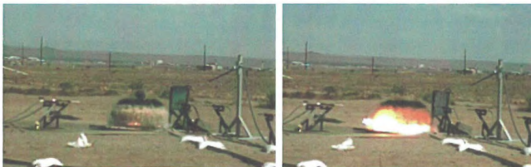
Figure 21: 0.8 lb of ██████/LH (left) and FGAN/LH (right) respectively at approximately t=625 μs.
