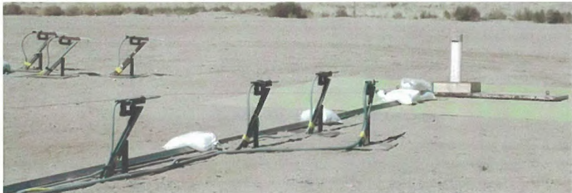
Figure 8: Pressure sensors placed at increasing distances from the charge.
