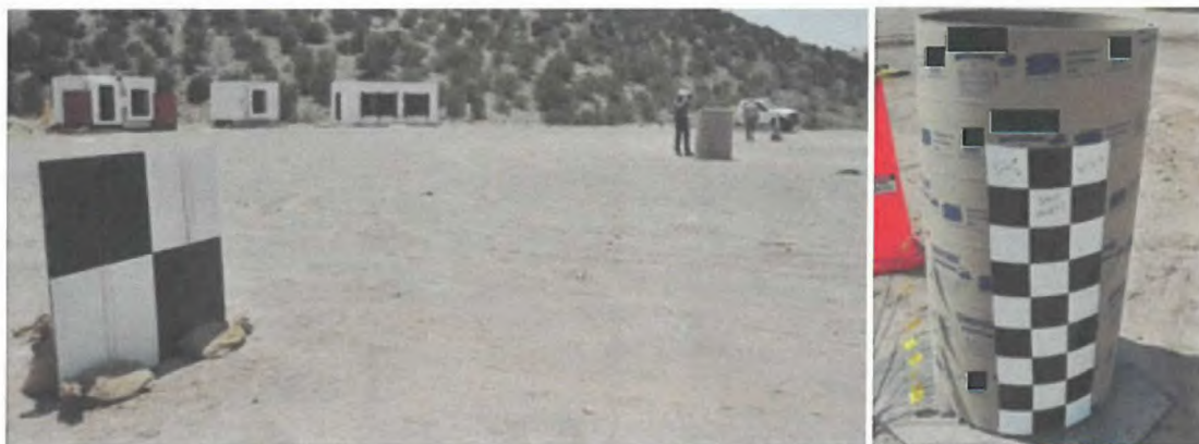
Figure 35: 3' x 3' Photometric fiducial boards were placed 50' left and right of the charge and fiducial sticker on charge container.
