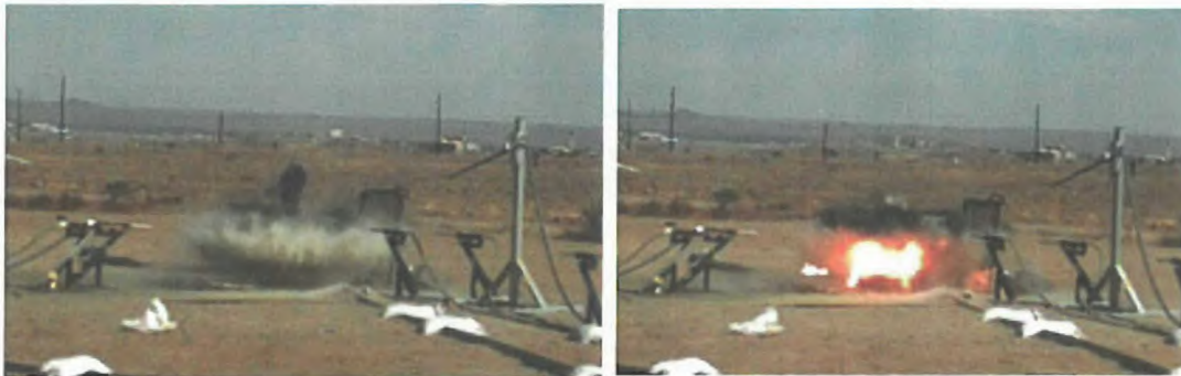
Figure 23: 0.8 lb of ██████/LH (left) and FGAN/LH (right) respectively at approximately t=2.187 ms.
