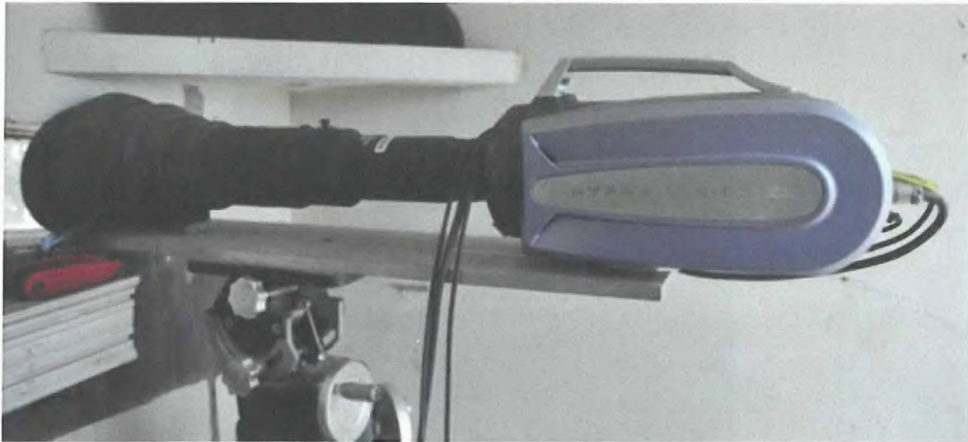
Figure 31: Shimadzu camera in the instrumentation bunker with long lens installed.
