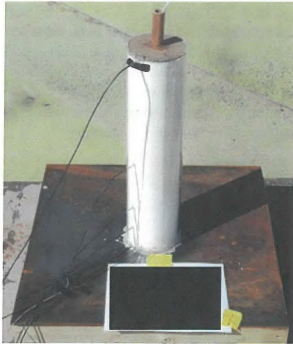
Figure 9: Time of arrival pins are inserted into the containment wall flush with the explosive material.
