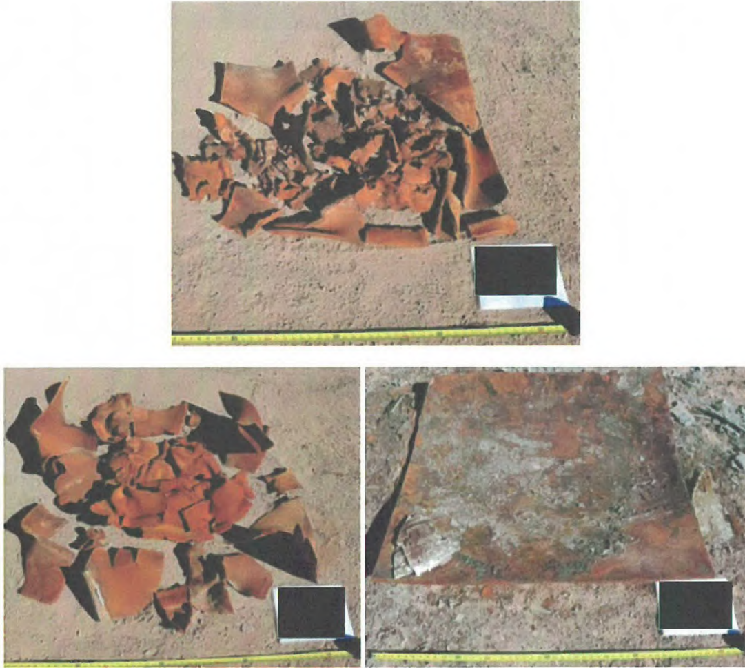
Figure 50: Witness plate damage from (top) commercial ANFO, (lower left) AN/AS 35.2/64.8 w/IP and (lower right) AN/AS 24/76 w/IP.
