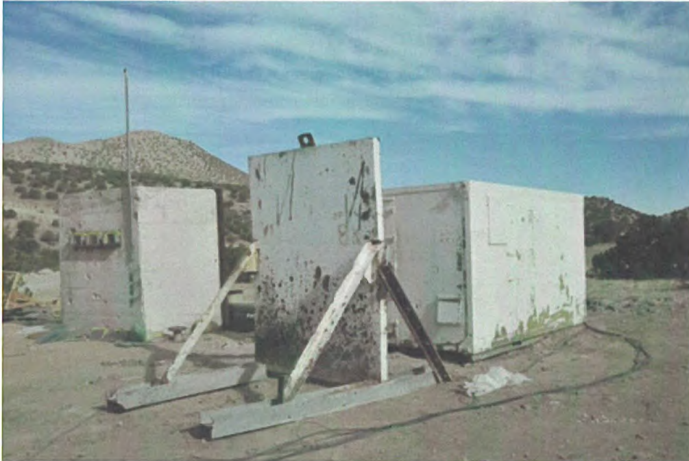
Figure 29: Instrumentation bunkers used to house and protect high speed cameras and oscilloscopes.
